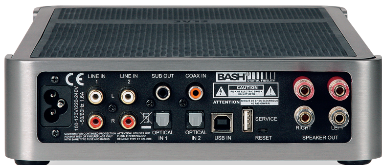
ABOVE: Two analogue line ins (internally sampled to 96kHz) are offered on RCAs alongside two Toslink optical, one coax and a USB Type B digital ins. A filtered sub out (RCA) and speaker outs (4mm) are joined by a USB Type A port for firmware updates
